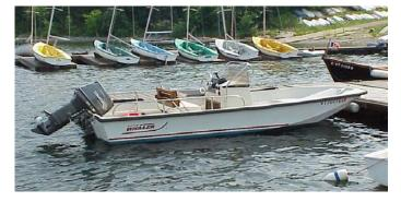
Bill Aldrich with a stand-up control console donated by Chris Morgan got together and a matching combination seat & storage locker, made repairs to the hull and replaced broken hardware and engine control. The result is a more modern utility boat that should be drier for its operators with more space for marks and their tackle.
